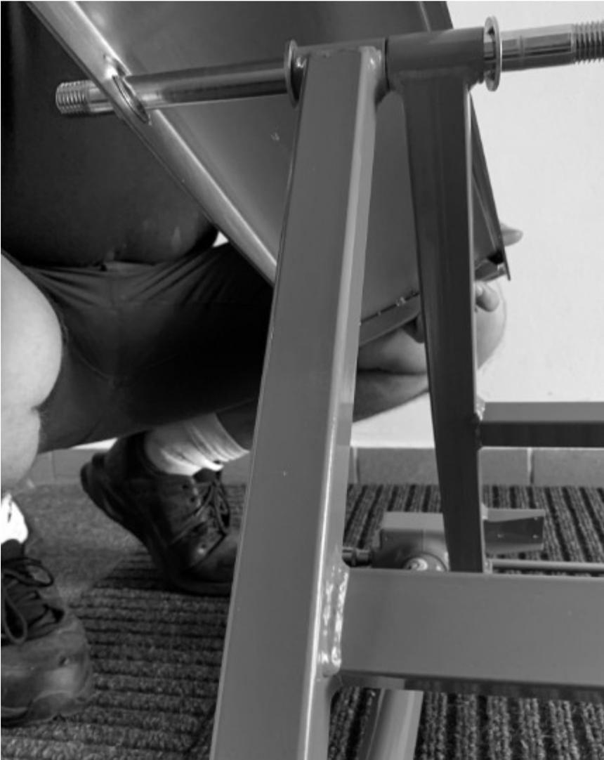
**Slide the bushings onto the axis bolt from both sides.**
