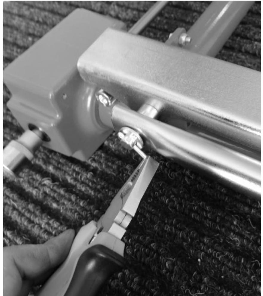
Place one of the rails for uneven surfaces on the lift, ensuring that the holes are accessible from both sides (do not be afraid to push the rail with force).
