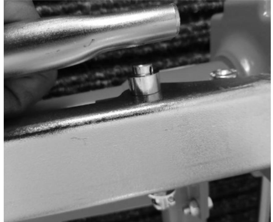
Slide the safety system tube back onto the pin, add the flat washer and re-secure it with the cotter pin.
