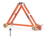
Place the tube between both holes and secure with pin, washer and split cotter pin.
